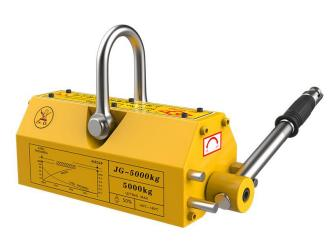
Magnetic Lifter 500kg, also known as magnetic chuck, is a magnetic fixture widely used in machinery factories, mold factories and other machining fields, which can greatly improve the clamping efficiency of magnetic steel materials. Magnetic Lifter 500kg is based on high-performance rare earth material Ndfeb (N>40) as the core, by hand pulling the handle of the chuck rotation, so as to change the magnetic system of ndFEB inside the chuck, to be processed to hold or release the workpiece.
