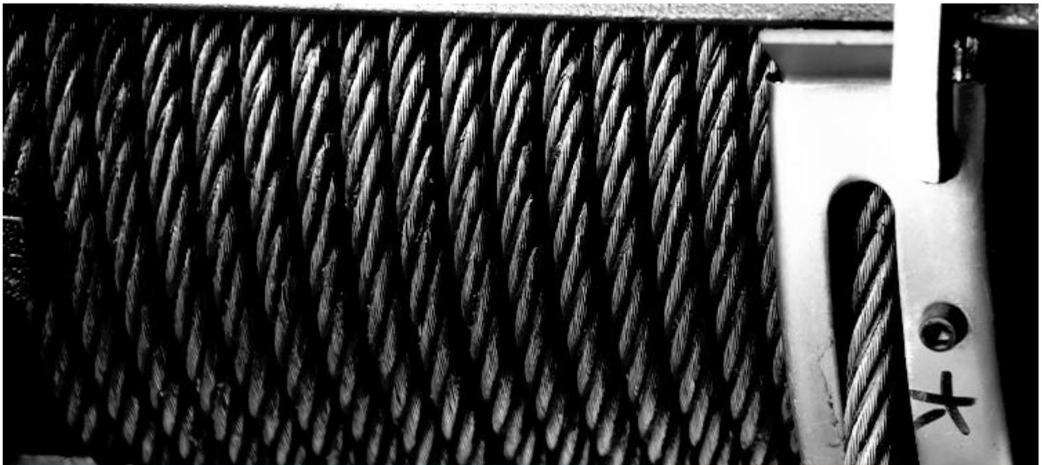
Electric cable hoist uses double flange drum cover, can effectively prevent wire rope winding to both ends of the reducer, prevent wire rope disorderly coil disorderly.
